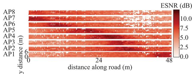
Figure 10: Effective SNR heatmap measured at each AP. In each heatmap the x-axis refers to distance along the road, y-axis refers to distance across the road. The AP radio coverage overlaps by between 6 m and 10 m.
