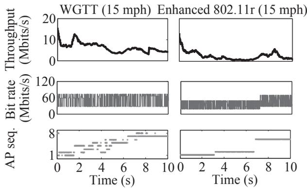
Figure 15: UDP throughput of WGTT and Enhanced 802.11r during a single client's 15 mph drive.
