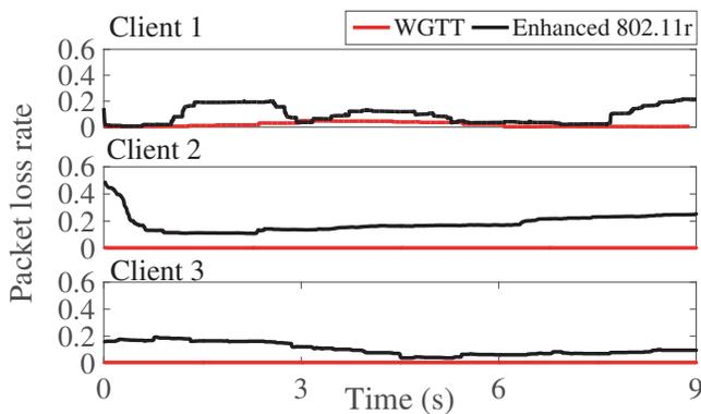
Figure 18: Packet loss rate of uplink UDP packets sent by three mobile clients.
