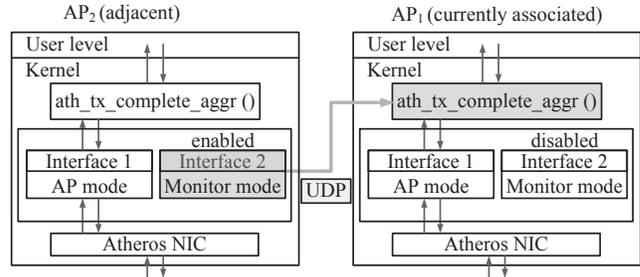
**Figure 8: WGTT's Block ACK forwarding design.**
