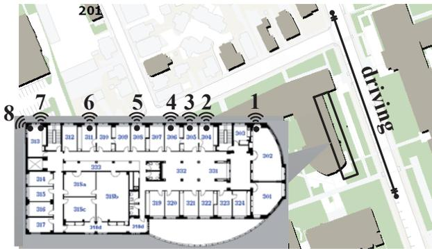
Figure 9: Experiment setup: we deploy eight WGTT APs on the third floor of an office building overlooking a side road with speed limit 25 mph. The radio coverage overlaps between adjacent APs.
