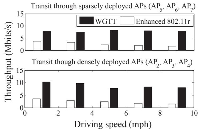
Figure 23: UDP throughput in areas of different density in our testbed deployment.
