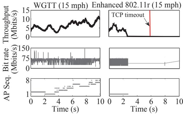
Figure 14: TCP throughput of WGTT and Enhanced 802.11r during a single client's 15 mph drive.
