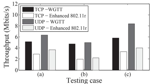
Figure 20: TCP/UDP throughput in different multi-client testing case. The client moves at 15 mph.
