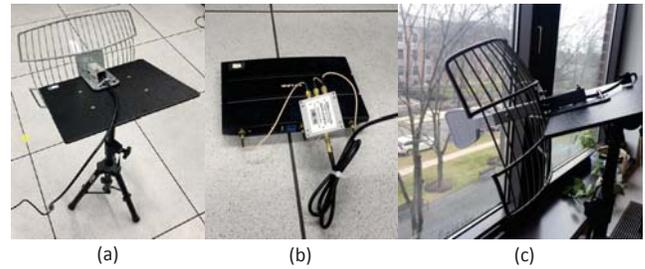
Figure 11: The WGTT AP is composed of (a) a directional antenna that connected to three ports of TP-Link AP via a splitter (b). (c): the AP is deployed in front of a window.
