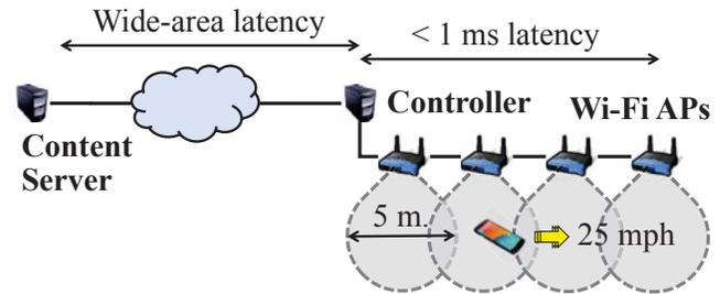
**Figure 3: *Wi-Fi Goes to Town* architecture: cars moving at 25 mph spend about 460 milliseconds in each AP’s cell.**
