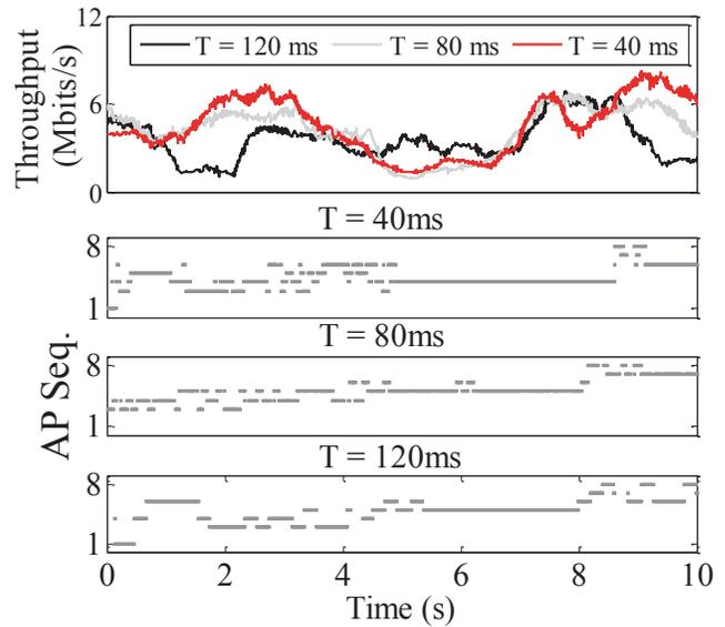
Figure 22: The TCP throughput against time in different and a timeseries showing which AP the client is associated with during its movement. The client moves at 15 mph.
