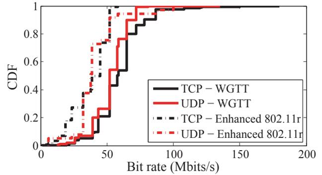
Figure 16: CDF of the link bit rate of TCP and UDP transmission. The client moves at 15 mph.
