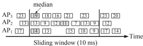
Figure 6: WGTG AP SELECTION: Choosing between three nearby APs, Wi-Fi Goes to Town examines the median ESNR reading from each, selecting in this case AP<sub>3</sub> with the greatest median SNR.
