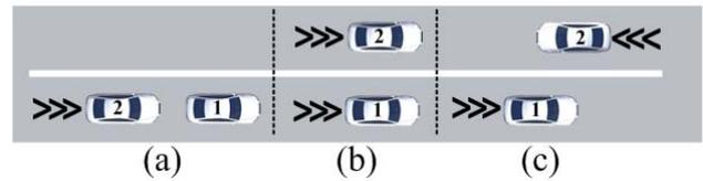
Figure 19: TCP/UDP throughput measurement testing in multiple client scenario, including (a) following driving with a spacing of 3 m; (b) parallel driving, and (c) driving in opposing direction. The clients move at 15 mph in each experiment.
