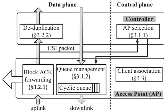
Figure 5: WGTG’s high-level design, divided into control plane- and data plane-functionality.
