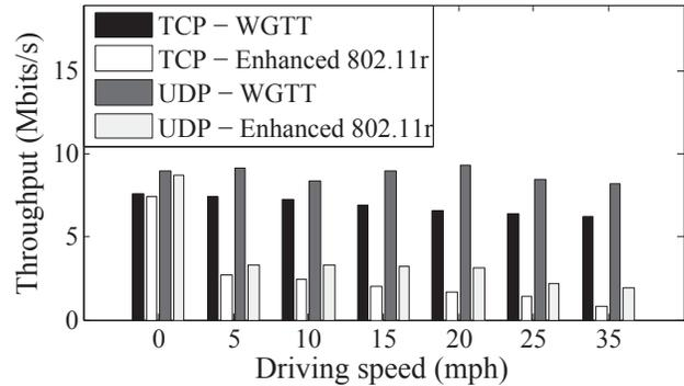
Figure 13: TCP and UDP throughput when the client moves at different speeds.
