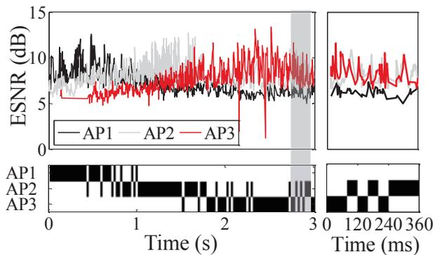
**Figure 2: THE VEHICULAR PICOCELL REGIME: Constructive and destructive wireless multipath fading as measured by Effective SNR (*upper plot*) conspire with vehicular-speed mobility to change the AP best able to deliver packets to a mobile client (*lower plot*) at millisecond timescales (*right detail view*). The radio coverage between APs overlaps by around 10 m.**
